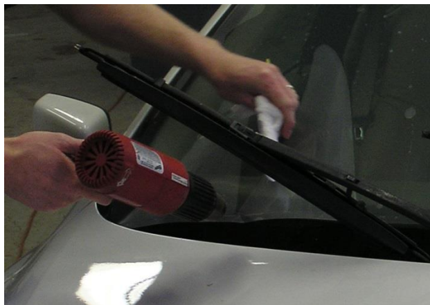
Figure 4 - Heat shrink film to surface
