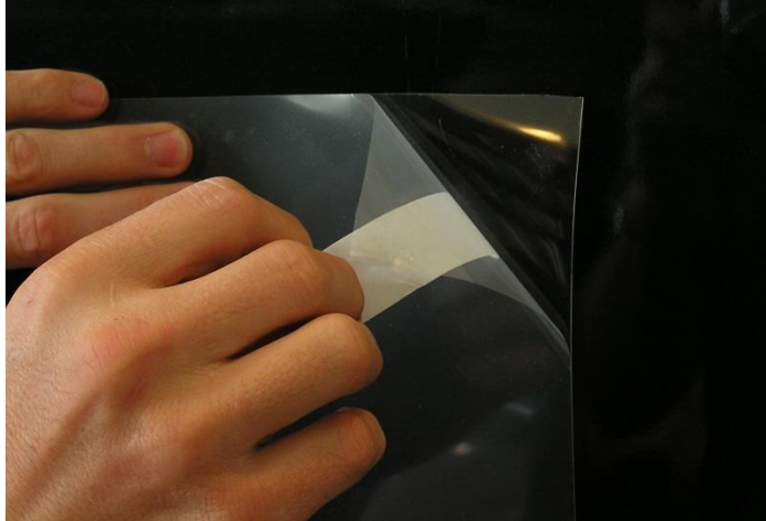
Figure 5 - Adhesive liner removal
