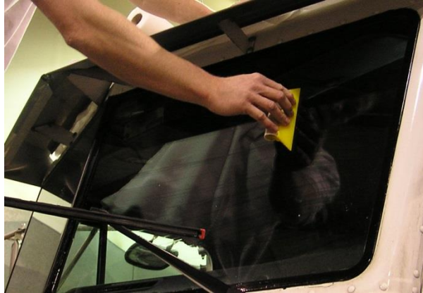
Figure 2 - Remove cleaning solution with squeegee
